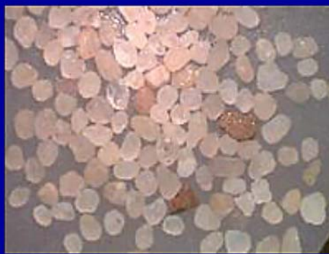
Figure 1, Clockwise: Trailers of sand and compressor trucks around a well during a hydrofrac job. Lower right, well rounded pure quartz sand typical of Wisconsin Cambrian sandstones. Lower left, basic principles of hydrofracking. Fracturing low permeability gas bearing shale with fluid pressure, sand is injected as a proppant to hold fractures open and allow gas to flow from rock.
